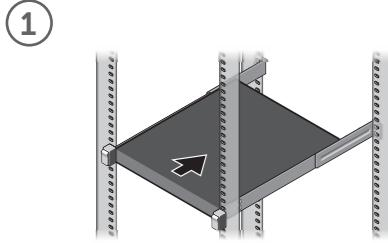
Install the system into a rack.
